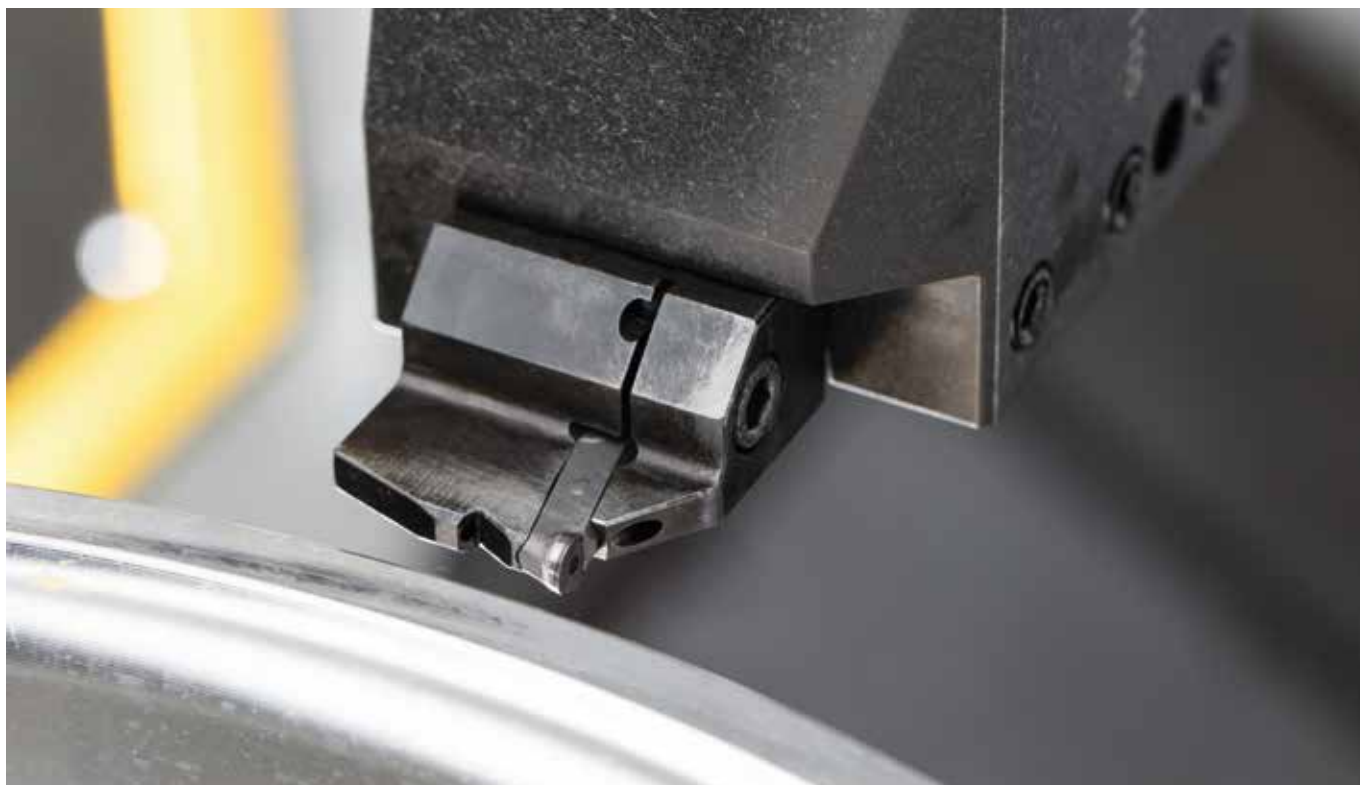
Turning the wheel flange with the S29F system.
