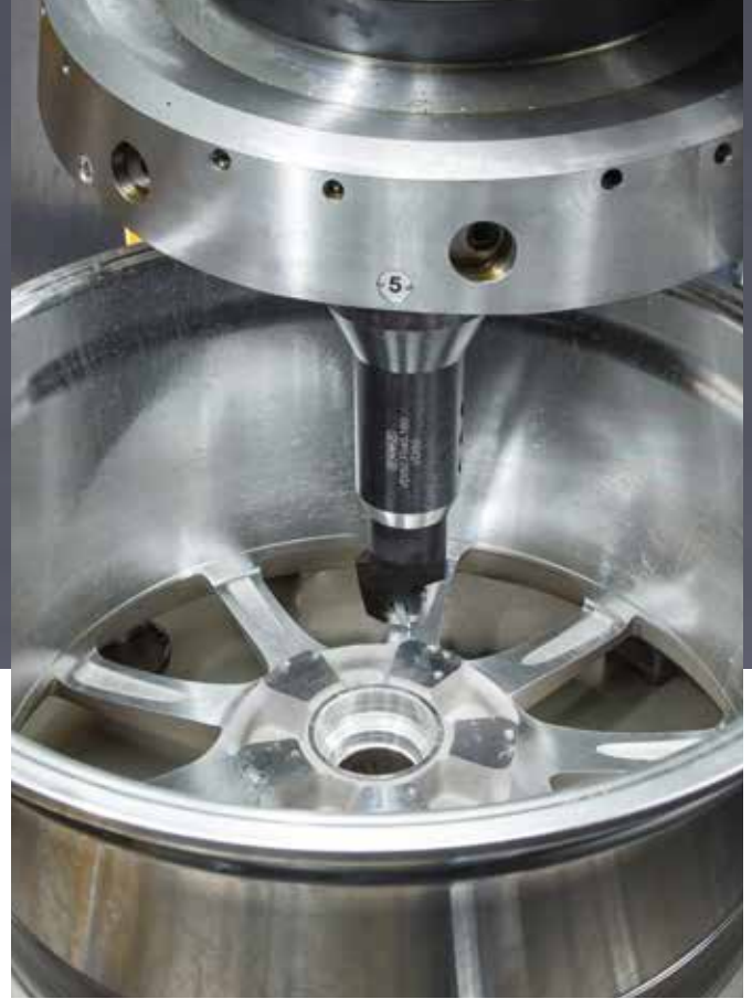
Turning the spokes with interrupted cutting.
